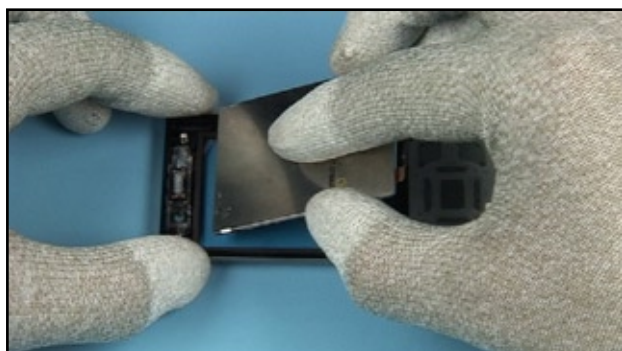
20. Place the LCD as shown.
